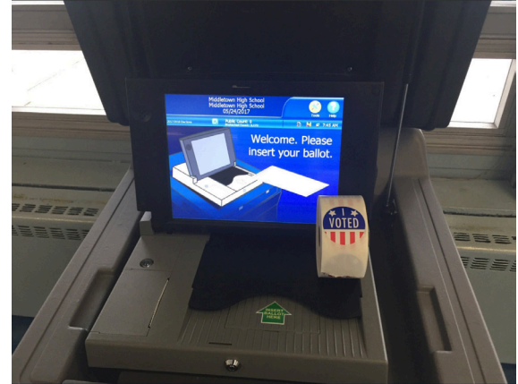
DS200 voting machine with new green arrow to better indicate where to insert ballot.
